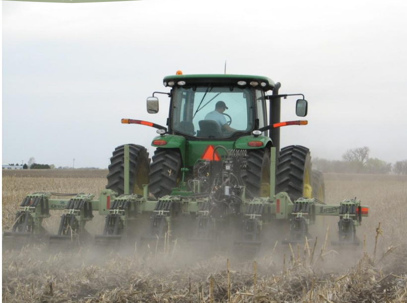
Orthman 8row Research Testing Unit – putting down pre-plant fertilizer
