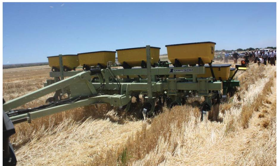
**Strip tillage makes it possible to plant directly into thick plant residues.**
